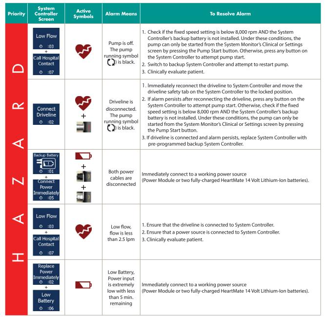
Important! The pump running (()) symbol is always lit green when the pump is running.
