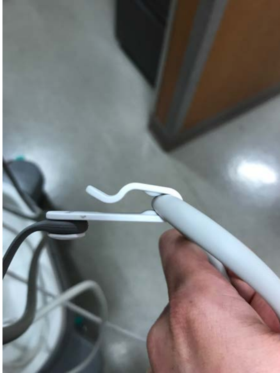
Hook Cords into the Clips to keep them out of the way of wheels
