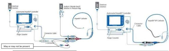
Correct configuration of the Impella system (2.5, 5.0, CP)
